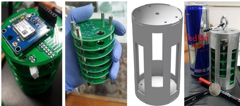
Views of Final Assembly of CanSat Built during above Workshops (Patents Filed)
