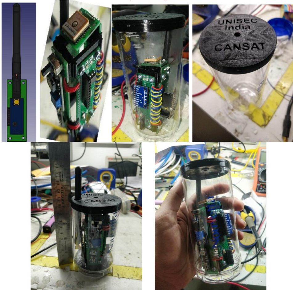
3D Printed Compact CanSat (Vertical Stacking of Boards Around Battery) (Patents Filed)
